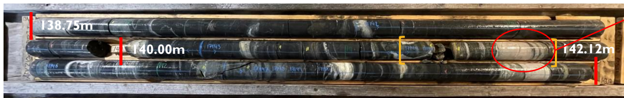
AEX21007, 141.14m – 141.69m (0.54m at 34.83g/t Au) Main Vein auriferous quartz vein intersection
