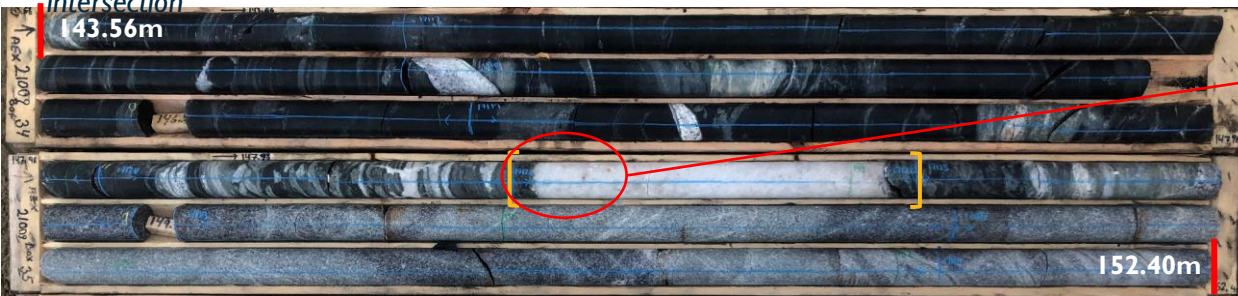
AEX21009, 148.57m – 149.08m (0.51m at 8.48g/t Au) Main Vein auriferous quartz vein intersection
